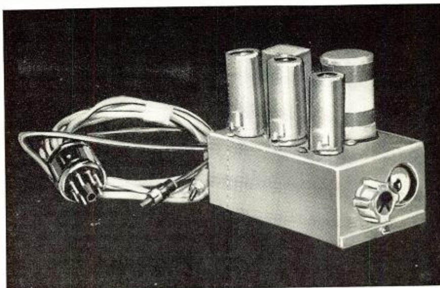
Over-all view of unit with level control and recording level indicator at front end. Shielded cables to record and erase heads and the power cable may be seen here. The tubes, filter capacitor, and bias-oscillator transformer are atop the chassis.
